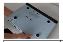
Turn the device upside down and then turn the screws in firmly.
