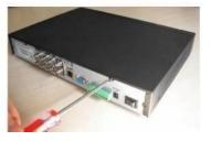
8. Secure the screws in the rear panel and the side panel.
