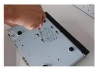
5. Attach the HDD firmly.
