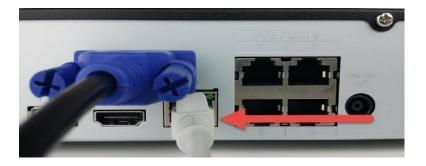
3. Connect the USB mouse to a USB port on the NVR.
