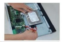
Connect the HDD cable and power cable.
